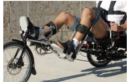
Orthoses provide a safe foothold. The speed is regulated using a "throttle".
